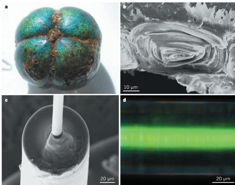
**Figure 1 | Fruit-inspired optical fibres.** **a**, The fruit of the tropical plant *Margaritaria nobilis* without its capsule (about 10 mm in diameter). **b**, Cross-section of the fruit seed coat shows a concentric, multilayered cellular structure. **c**, Cross-section of a soft multilayered optical fibre around a glass core, fabricated by Kolle and colleagues<sup>3</sup>. **d**, Reflected green colour from the soft optical fibre in **c**.
